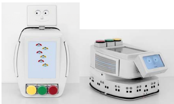
Fig. 2. Vertical (left) and horizontal (right) configuration
