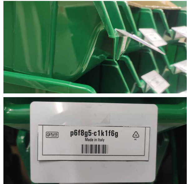
Fig. 4: Detail of the standard storage bin with a labeled NFC card.
