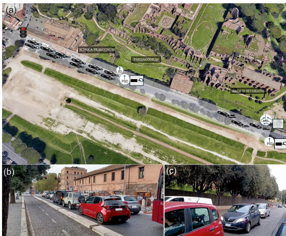
Fig. 7. (a) Grain-size model of the vehicular emissions at Via dei Cerchi: car queues from the traffic light to the Paedagogium and Schola Praeconum sides of the road: prevalence of Single Domain (SD) and Pseudo Single Domain (PSD) fine particles connected to exhaust emissions (modified from Google Earth). Smooth traffic conditions at the Arcate Severiane side of the road mixture of MD and PSD particles respectively connected to brakes and fuel emissions.
