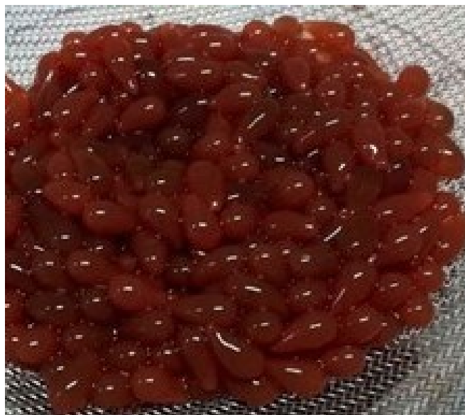
Figure 6. CMC-5 hydrogel beads show dark color due to the presence of \text{Fe}^{3+} ions in the polymer network.
