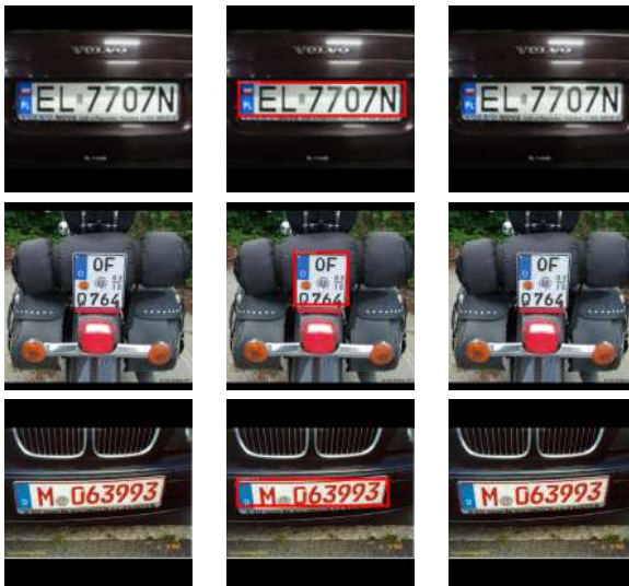
Figure 8: Each row illustrates, from left to right: the original (clean) license plate image, the corresponding detected license plate region, and the adversarial example generated using the I-FGSM attack, restricted to the license plate area.
