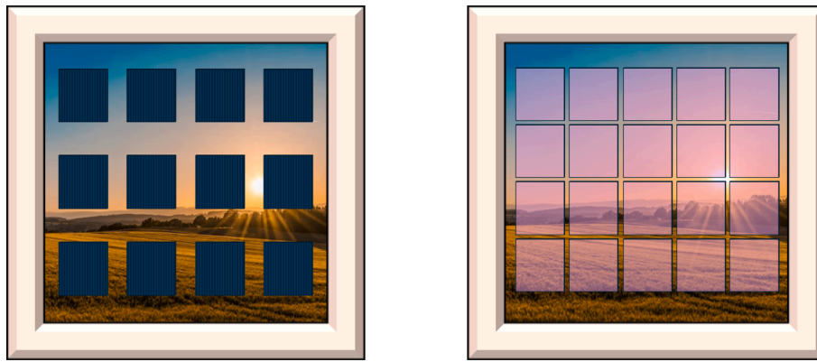
Fig. 2. Schematic representations of ST-PV glazing systems with opaque solar cells (OP-SC)(on the left) and semi-transparent solar cells (ST-SC) (on the right).
