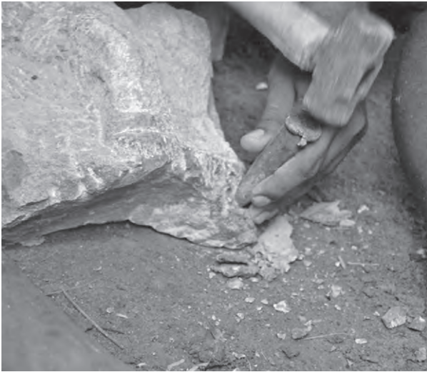
Figure 4.4. Hammering of a granite block with a steel point in Mahabalipuram, India. Photo: Haris Procopiou.
