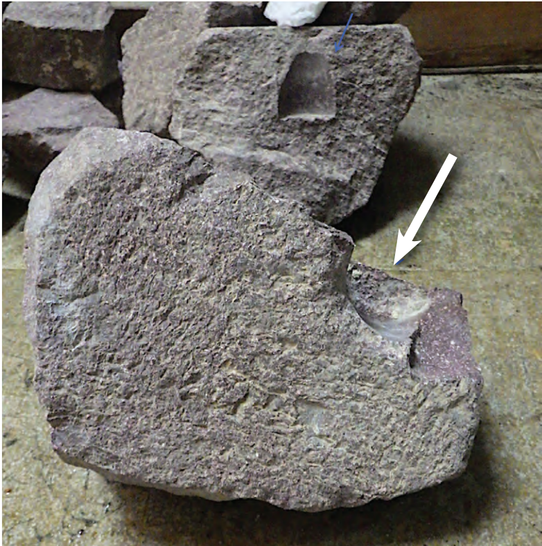
Figure 4.5. Blocks of porphyry with cavities drilled using a tubular drill (cathedral of Monreale). Photo: Élise Morero.
