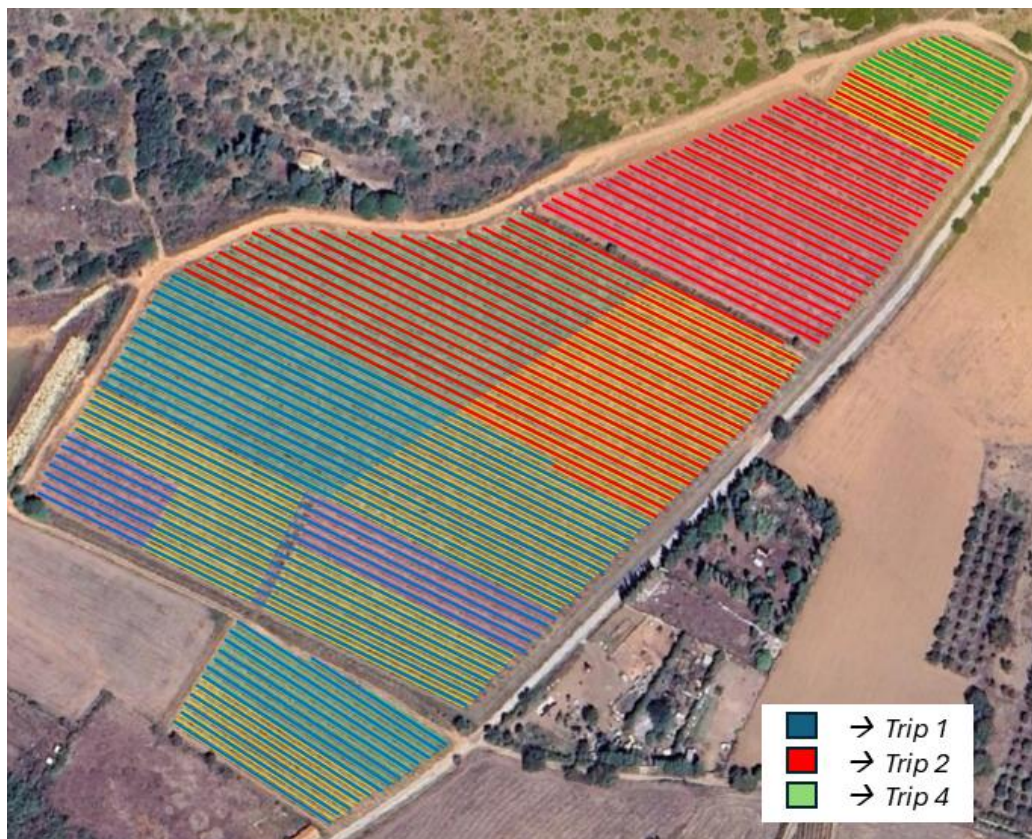
Figure 2.3: Treatment of Field 1 in Trip 1, 2 and 4 as proposed by the Post-processing algorithm. In each trip, where Field 1 is visited, a specific number of rows must be covered, including a final row that is only partially treated. Rows highlighted in blue, red, and green represent Trip 1, Trip 2, and Trip 4, respectively.
