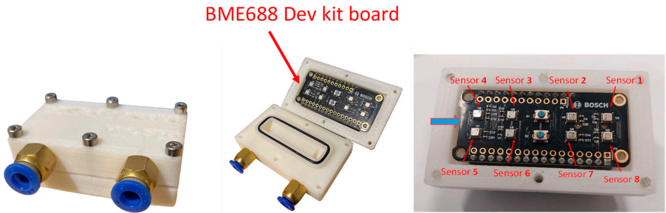
Figure 1. Gas sensor measurement chamber shown in both closed and open configurations, with the BME688 Development Kit housed inside, which embeds the 8 identical BME688 gas sensors.
