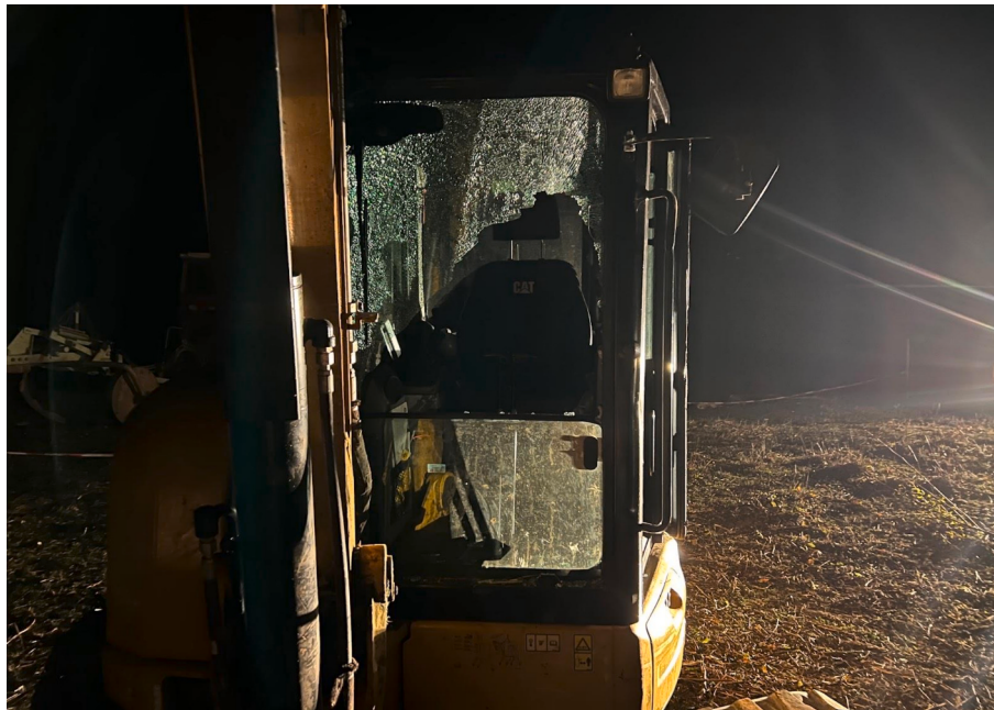
Photo 2. The front windshield was shattered and missing its lower-left portion.
