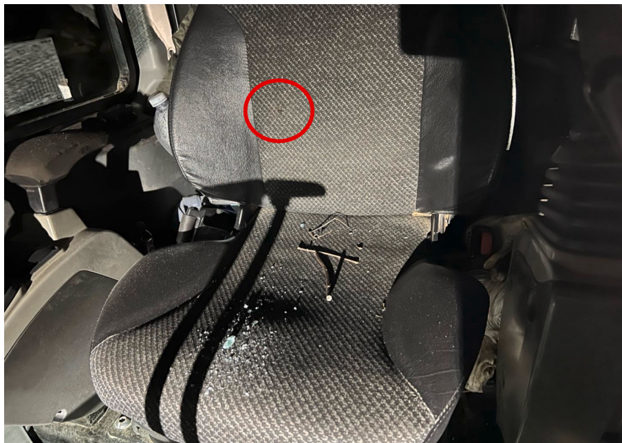
Photo 3. Metal fragment and glass fragments on the seat. On the upper left part of the backrest, a small hole in the fabric.
