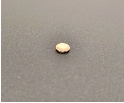
Figure 4.6: Solid target of 99.9% pure silver
