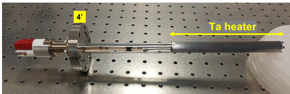
Figure 6.6: Effusion cell WEZ40-5-16-D16-standard, to be connected through port 4' of the reaction chamber. The right end has an opening through which the crucible is placed inside the Ta heater.
