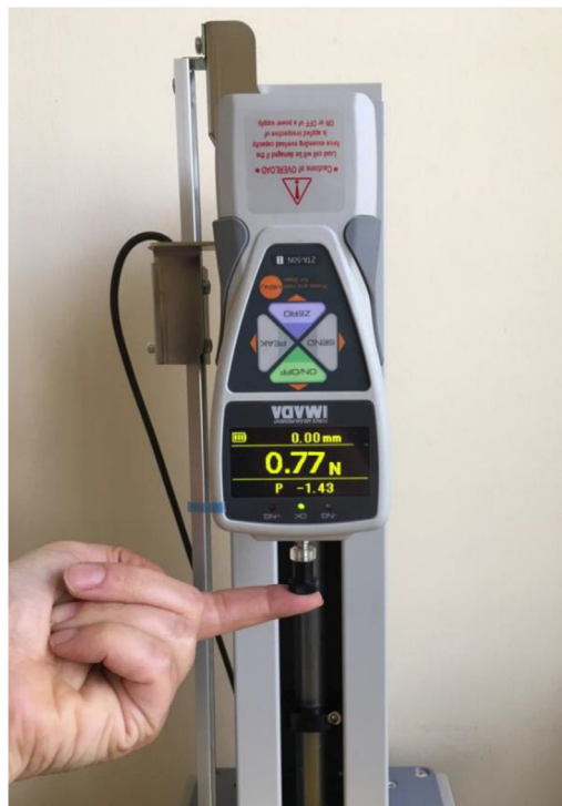
Fig. 9. Force-displacement tests with digital transducer.
