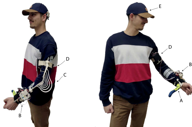
Figure 2.7: The Robotic Sixth Finger (A) and its power supply and control system (B), developed by US, has been integrated with the Assistive Elbow Orthosis (C), developed by UT, and the CUFF (D) from UP. The CUFF has been modified to be completely wearable. Motion of the finger is controlled via a new e-Cap version (E) developed by US with novel 3D-printed electrodes by UT
