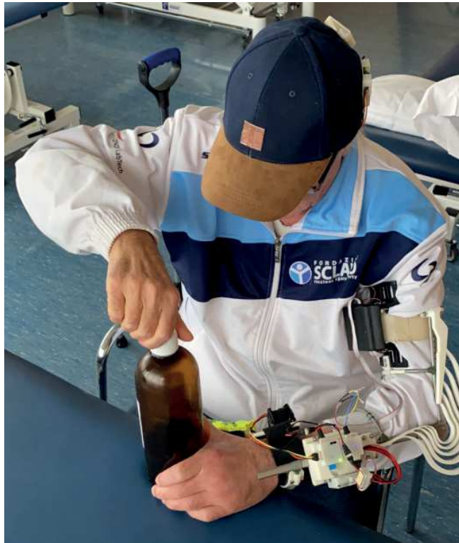
Figure 2.8: A stroke patient opening a bottle with the help of the SoftPro Wearable System.
