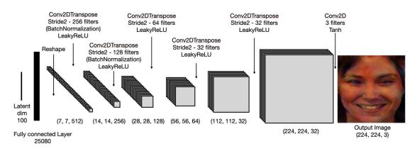
Figure 3. Generator architecture
