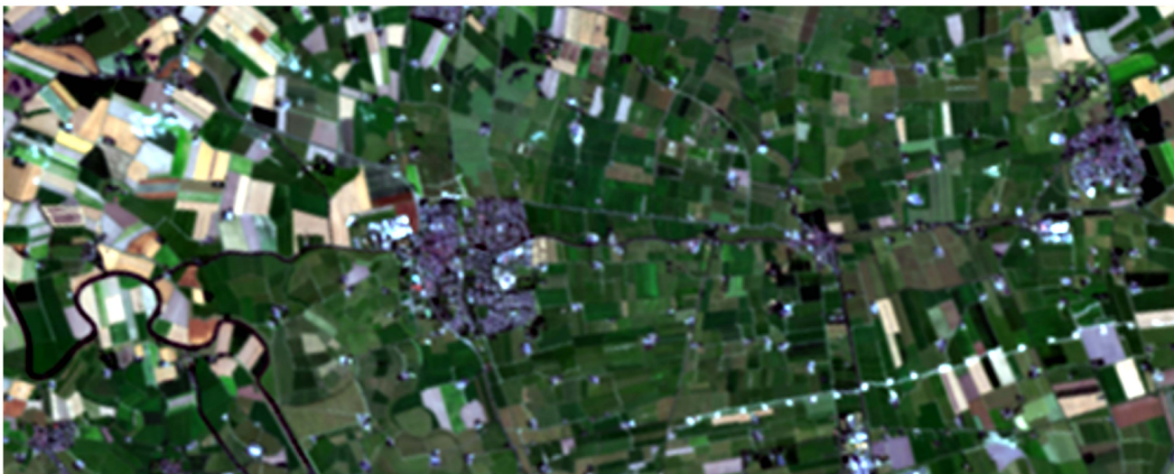
Fig. 4. 15 km \times 6 km EnMAP acquisition: (647-551-468) nm composition at 30 m spatial resolution, interpolated at 10 m.
