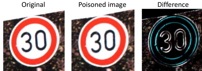
Figure 3.3: Poisoned image based on image warping. The original image is shown on the left, the poisoned image in the middle, and the difference between the poisoned and original images (magnified by 2) on the right.
