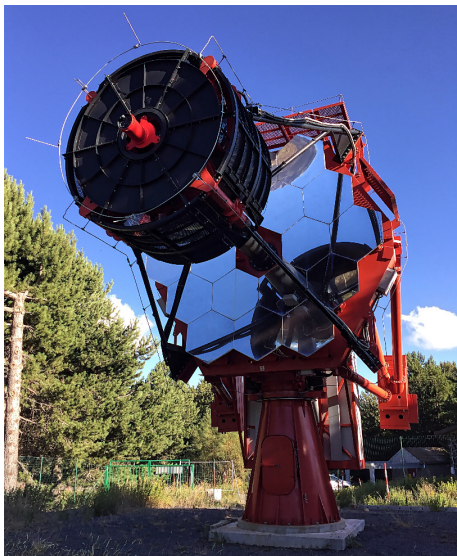
Figure 4. The ASTRI telescope and its dual mirror optics [26]. Reproduced with permission, Copyright ESO.
