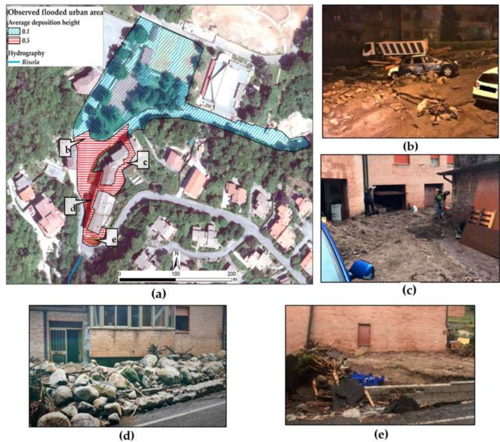
Figure 5. (a) Aerial view of the urban area impacted by the debris flow deposition in Via Fosso Canali; (b–e) deposition of debris in the inhabited area with the involvement of houses and cars (Sources: (b,c,e) Unione dei Comuni Amiata Val d’Orcia; (d) [42]).
