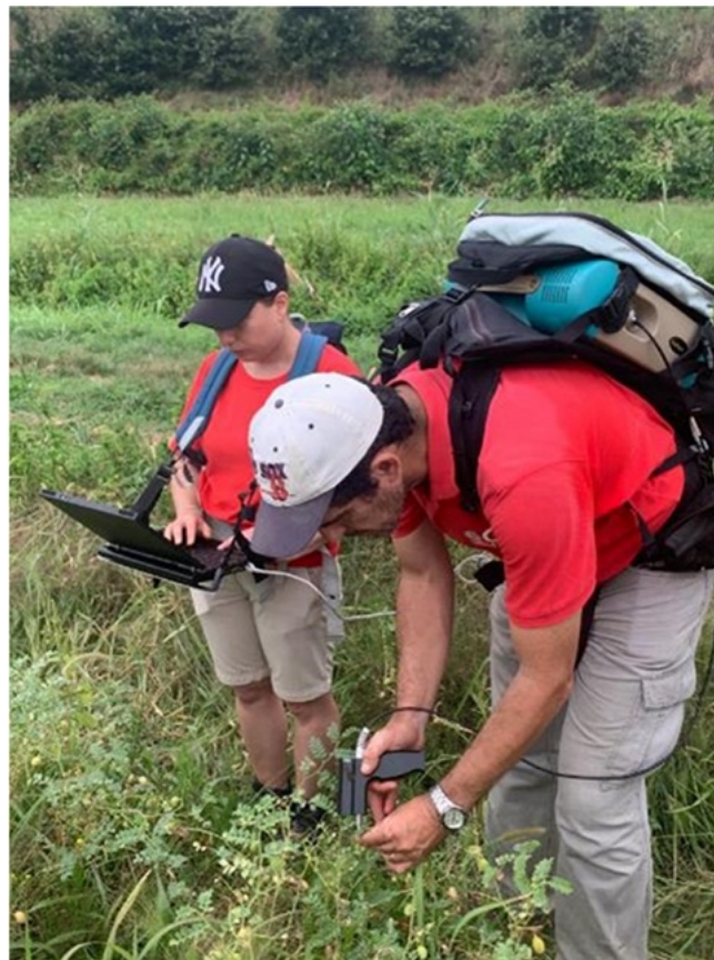
Figure 7. Acquisition of spectral signatures during fieldwork. For each plant, an adaxial side of the terminal leaflet of the five youngest fully expanded leaves and the surface of a fully developed pod (green in color and full of seeds) were considered.
