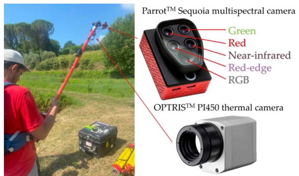
Figure 4. Setting of the Parrot™ Sequoia multispectral camera and Optris™ PI450 thermal camera on the support.
