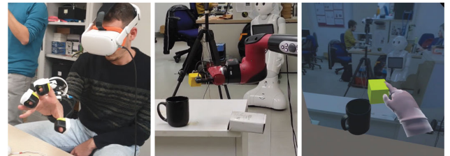
FIGURE 10. Experiment 2. The user immersed in the augmented environment picks and places a soft yellow cube simulating a fragile object. The force data are acquired by the ATI sensors integrated on the robot gripper, and reproduced by the haptic interface on the fingers of the user.
