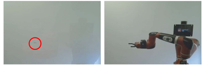
FIGURE 9. Experiment 1. Comparison of frames after (left panel) and before (right panel) applying the robot concealment algorithm. The residual pixels that contain the robot after the concealment are red circled in the frame on the left.
