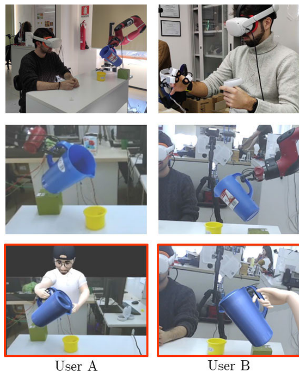
FIGURE 1. Physical Metaverse representative scenario. Two users (User A and User B) are in different locations and can interact in a shared environment of the metaverse, which is an augmented version of User A's physical surroundings (top left panel). Through a head-mounted display, User A observes his workspace (middle left panel) diminished of the robot, and augmented with the digital twin of the pitcher and the virtual avatar of User B (bottom left panel). At the same time, User B (top right panel) observes the same environment from a remote camera that streams into his head-mounted display (middle right panel). The robot is removed from the video stream and substituted with User B's virtual arm (bottom right panel). User B controls the Avatarm, hence can manipulate real objects in the physical environment of User A and feel the interaction through a wearable haptic interface.
