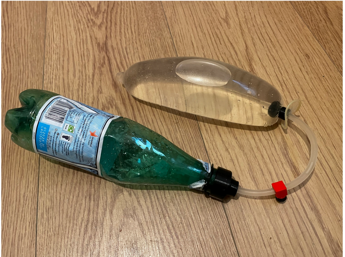
Fig 2. The setup of the open-air experiments: The condom filled with water and the flow-stopper that prevents the water from flowing back through the tube.
