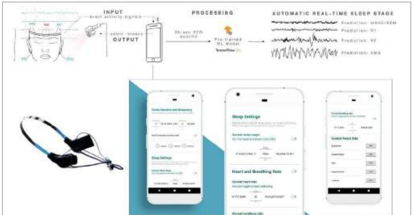
FIGURE 5 | The system reads brain activity signals and sends this information from the EEG to the smartphone via Bluetooth Low Energy (BLE). The app integrates a pre-trained machine learning model that takes 30 s worth of data from the EEG and predicts a sleep stage with a given accuracy. The user or experimenter can customize the duration and frequency of the olfactory stimulation in certain sleep stages using the smartphone app. Scent can be activated manually using a button, or automatically based on physiological signals, such as heart rate and breathing rate. The system can also release scent based on the user's sleep stage, or based on time, e.g., 20 min after going to sleep.
