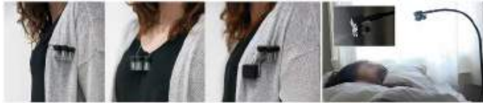
FIGURE 3 | Ezzence can be worn during the day and be attached to a bedside holder at night. It can also hook onto pajamas, blankets, necklaces or, inspired by a brooch; each part can be attached separately. The custom holder charges the device and has an adjustable flexible neck. It wirelessly connects to the smartphone application that controls the duration and frequency of the scent bursts and activates odors depending on physiological signals, sleep stage, and the user's preferences.
