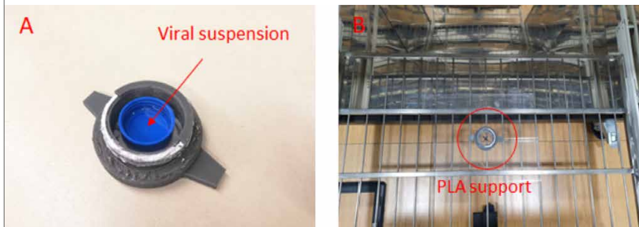
Fig. 3. (a) the PLA support (grey part) used for the test. Inside the support, the viral inoculum has been placed in a plastic test tube cap (blue cap). (b) Placement of the PLA support on the metal grid of the device (view from above).
