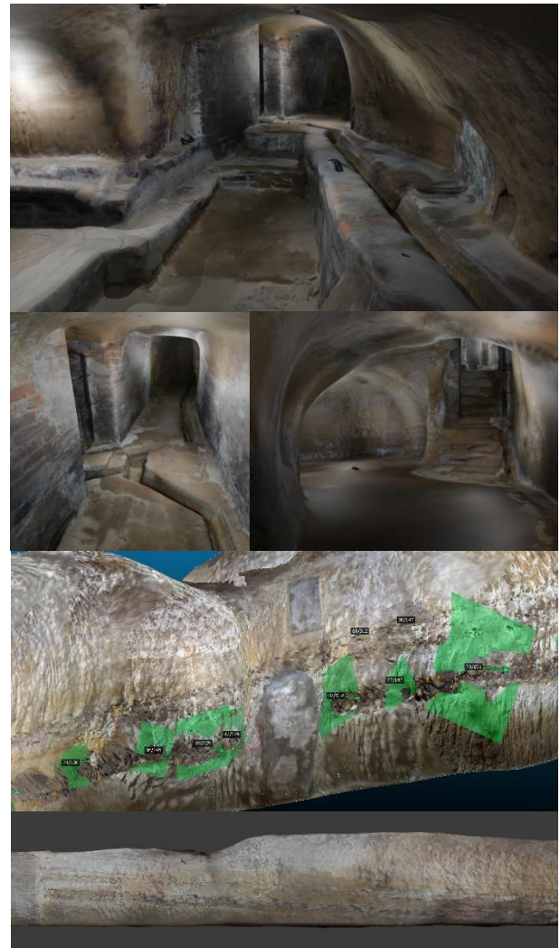
Figures 5 a-b-c-d-e: (a-b-c) rendering of the detected sector of Figure 4a; (d-e) 3D reconstruction of the geological model of a surveyed section with identification of the geological limits between the sands and the gravels, and their consequent orientation in space
