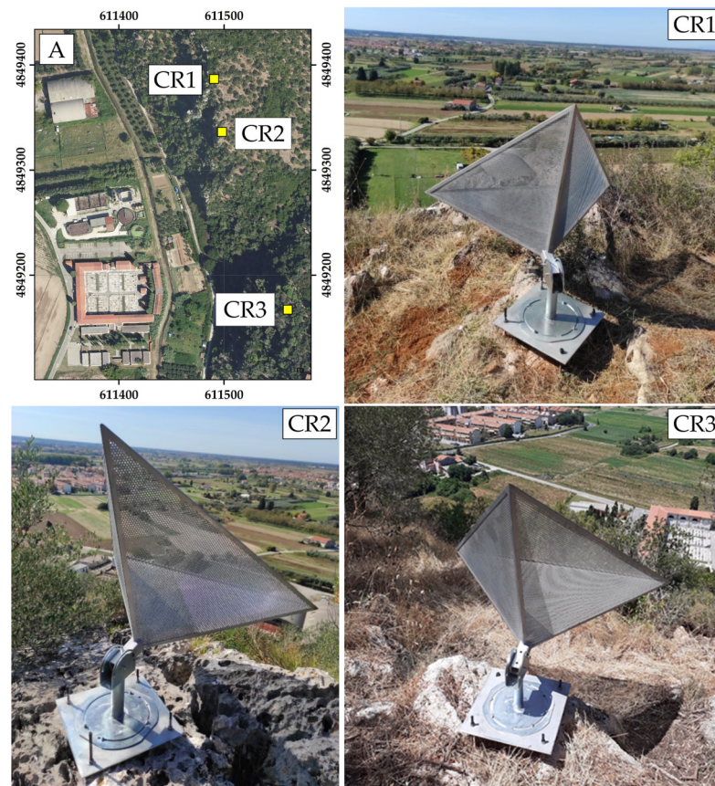
Figure 3.55: Metallic corner reflectors positioned along the upper edge above the rock walls: (A) map of reflector locations in the study area; photographs CR1, CR2, and CR3 illustrate detailed views of the installed devices.
