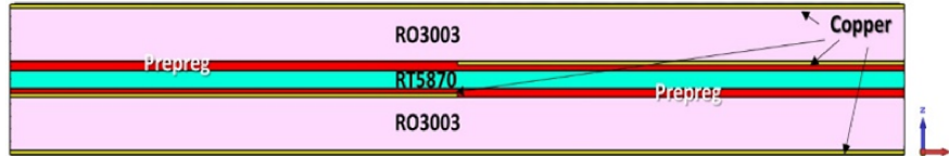
Figure 3.10: Stack-up of the prototypes.
