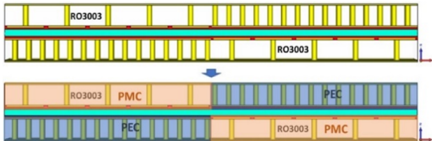
Figure 3.11: Transverse cross-section of the PTD-BEW. The prepreg is represented in red, copper in yellow, Rogers RT5870 in light blue. The bottom picture highlights the regions emulating the ideal PEC/PMC BC.
