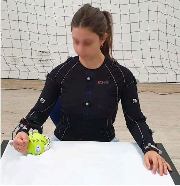
Figure 1. A user exploiting her Intrinsic Kinematic Null Space for controlling the opening/closing mechanism of a wearable robotic extra-finger in an augmented manipulation task. The task requires the involvement of natural (i.e., the right arm) and artificial (i.e., the robotic extra-finger) limbs to pick and place objects.
