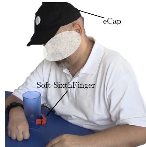
Fig. 1. The Soft-SixthFinger. The robotic extra-finger works with the paretic limb to compensate for hand grasp functionality. The patient can control the device thanks to a wearable EMG interface embedded in a cap called eCap.
