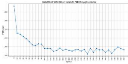
5(a) FID score progression of generated samples for each epoch. This metric quantifies the model's convergence and generative quality improvement.
