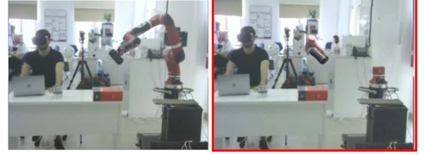
Fig. 1: Physical Metaverse representative scenario. On the left the scene captured by the real camera, on the right the scene as seen in the Physical Metaverse.
