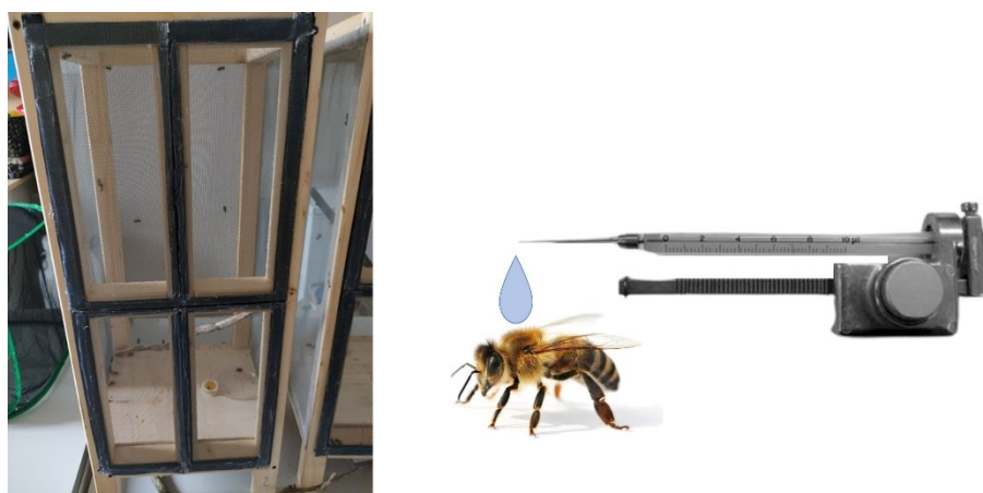
Figure 2. Cage used for the experiment and Burkard hand microapplicator equipped with a 1-mL syringe
