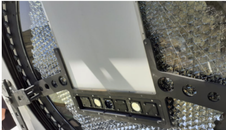
Figure 3.3.: Filter holder with room for up to six filters, fixed to the holder of the spectralon target. Two filters were installed (white circles) when the image was taken. One of the holes was left open and the three other ones were closed with a plastic cap. Behind the spectralon target, the Winston cones of the camera pixels are visible. Image credits: Juan Cortina.
