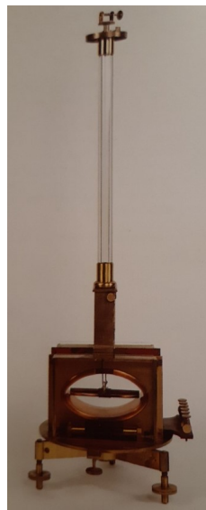
Figure 2.10: Weber's magnetometer (1832). Image courtesy: National Museum of Science and Technology "Leonardo Da Vinci" (Milan). Italy
