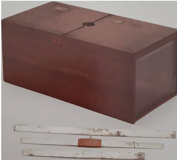
Figure 2.1: Prony's declinometer (1783 – 1820). Image courtesy: "Museum "Galileo", ex Institute and Museum of History of Science". (Florence, Italy)
