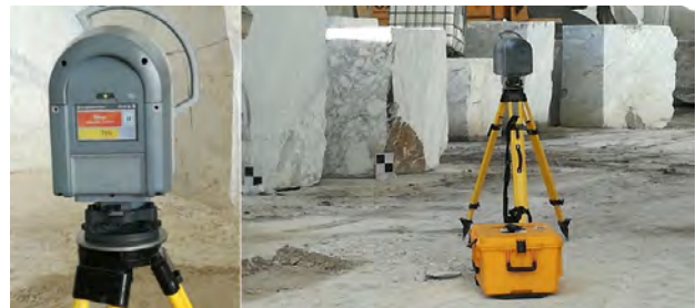
Fig. 4 - TLS at work in the “Piastraio di Sotto” quarry. Detail of the TLS during data acquisition (left). TLS and black and white targets, in background, used for data registration and georeferencing (right)
