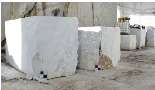
Fig. 6 - Example of the black and white targets positioned inside the quarry
