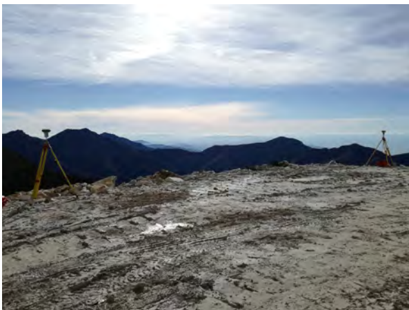
Fig. 5 - Dual frequency geodetic receivers operating in static modality in the areas facing the “Piastraio di Sotto” quarry entrance
