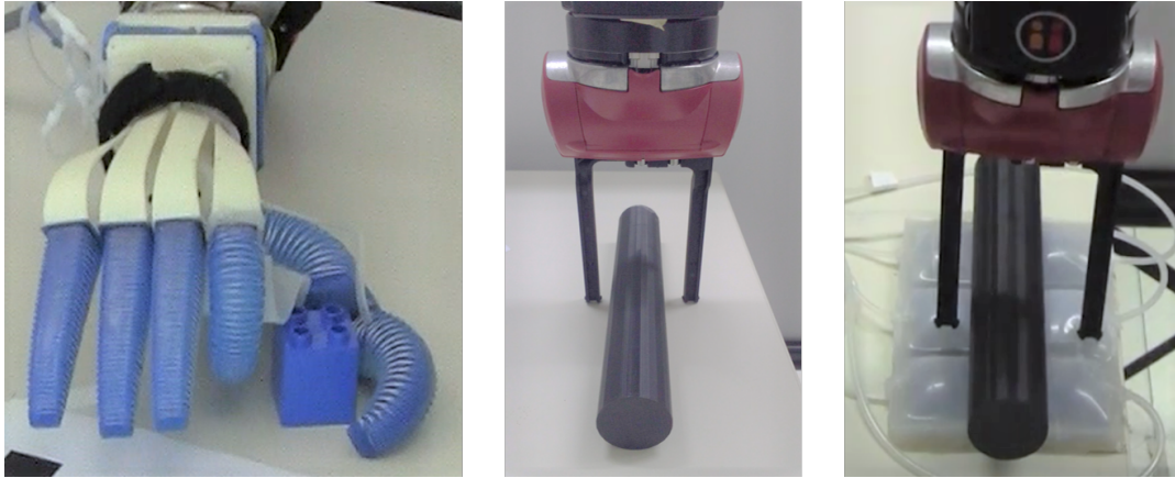
Fig. 4.37 Soft hands, like the RBO Hand 2 [196], can easily interact with rigid surfaces for grasping objects (left), rigid grippers, instead, cannot safely exploit the environment (center). We propose a soft sensorized surface (right) that allows rigid grippers to exploit the environment to pick objects up and provides a grasp planner with information on object pose and weight distribution.
