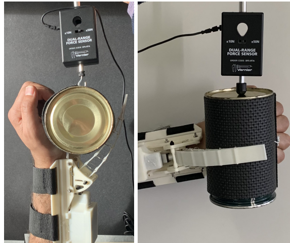
Fig. 3.21 Experimental setup for measuring the maximum payload and horizontal grasp resistive force.
