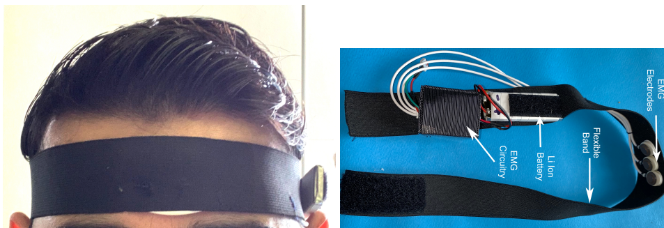
Fig. 3.19 Frontalis muscle based EMG interface to control the motion of the device. The EMG interface is embedded in a head band to improve its wearability and easy to use.
