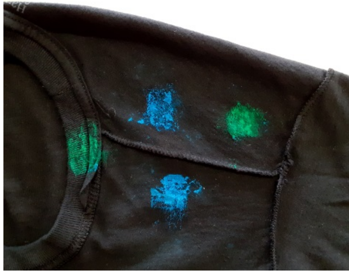
Fig. 4.34 Estimate of the fabric portion involved in the grasp, with and without the electromagnet exploitation (blue and green marks, respectively). A smaller portion produces fewer wrinkles, increasing the grasp precision.
