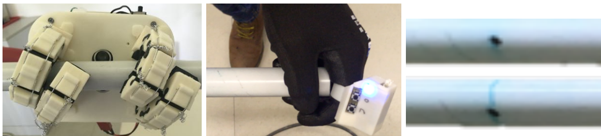
Fig. 4.15 Particulars of the collaborative task. On the left side, how the object is grasped using the reconfigurability of the fingers. On the center, the hand of the human operator together with the ring interface is shown. On the right hand side, the pipe before (up) and after (down) the operator drawing.
