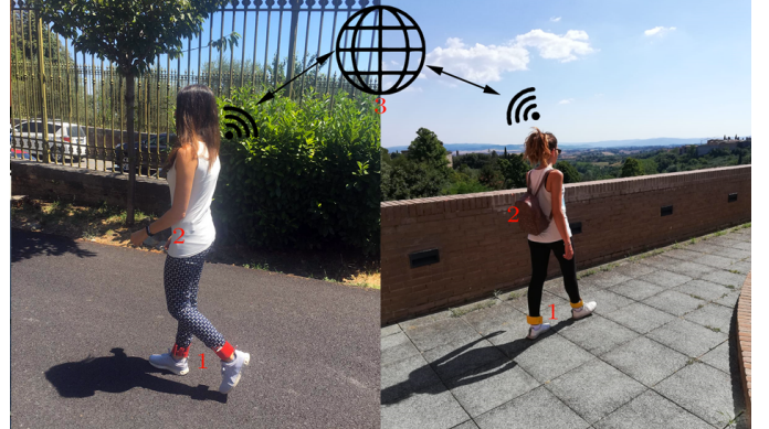
Fig. 1: The proposed remote social walking system: i ) the ankle device (1) measures user A gait cadence; ii ) the smartphone (2) receives the measurement via Bluetooth; iii ) the information is sent to a server via the Internet (3); iv ) the server sends the update to the user B ’s smart-phone; v ) the smart-phone (2) commands vibrations at the user’s anklets (1).
