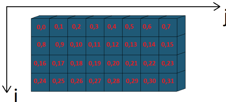
(a) Coalesced access with all the threads in the warp accessing contiguous elements in the same section.
