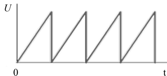
Figure 2. The Franck-Hertz device, showed on the left, allows to visualize the transmitted current directly on the screen of an oscilloscope if the tube was powered by a voltage U varying as a sawtooth wave (on the right).
