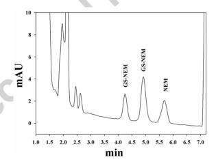
**Fig. 1.** Representative chromatogram obtained from a blood sample derivatized for GSH analysis. Blood from a healthy donor was collected in the presence of NEM. Sample was then deproteinized and supernatant was analysed by reversed-phase HPLC at 265 nm wavelength [61]. The GS-NEM
