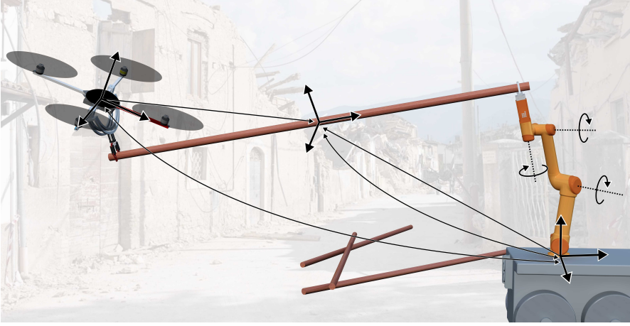
Figure 4.1: Representation of a MAGMaS, a heterogeneous multi-robot system composed by a ground manipulator and one aerial robot, in a USAR scenario. Overlaid are the main coordinate frames, states, and control inputs used in the dynamic modeling.
