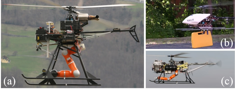
Figure 1.1: Examples of works in aerial manipulation with conventional helicopters with actuated robotic arms. (a) Aerial manipulation robot composed of an autonomous helicopter and a 7 degrees of freedom industrial manipulator [4], (b) small scale UAV helicopters with added payload mass [5], (c) visual servoing for aerial manipulation using a 7 degrees of freedom industrial manipulator [6].
