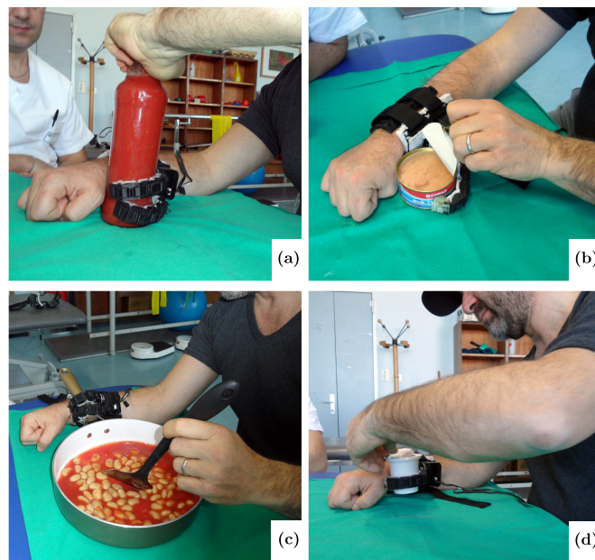
Figure 4.19: Preparing lunch with the help of grasping compensatory robotic device. (a) opening tomato sauce jar, (b) opening tuna can, (c) stirring food, (d) opening yogurt cup
