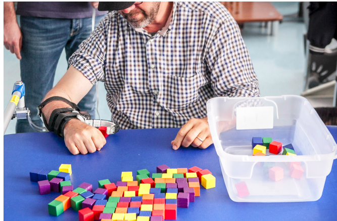
Figure 7.3: The box and block test: The subject grasped the object with the help of the soft-sixthfinger while using passive arm support to assist the paretic arm
