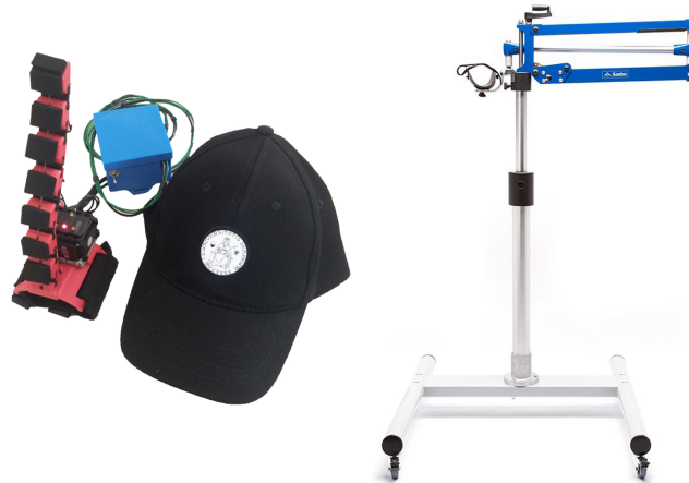
Figure 7.2: On left: Soft-SixthFinger, controller unit and eCap. On right: SaeboMAS for compensating the gravity of the arm.
