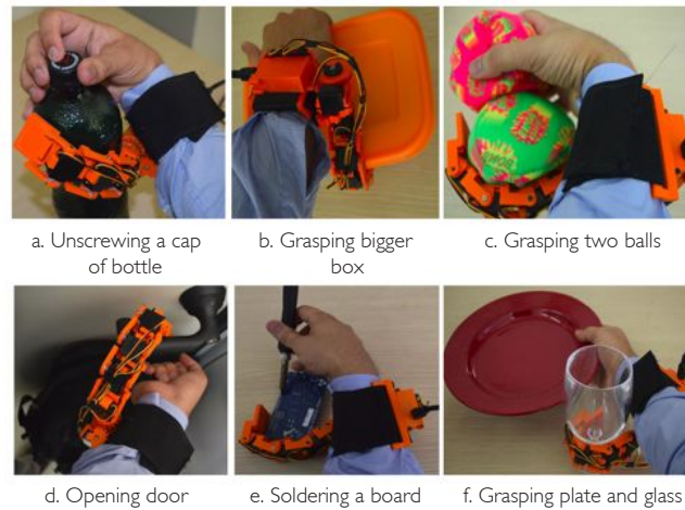
Figure 6.16: Examples of tasks performed by the augmented hand, i.e., human hand plus supernumerary robotic finger. In all the tasks, the human healthy hand and robotic finger work together to complete the tasks which are impossible to do with human hand only.
