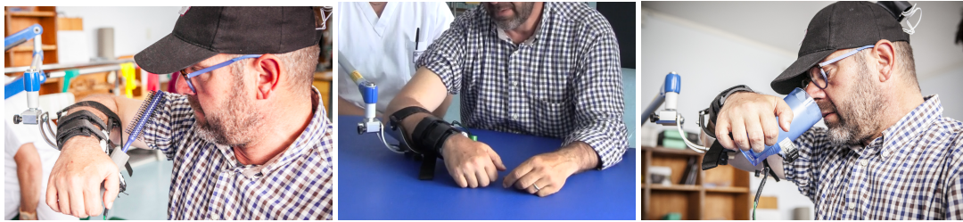
Figure 7.4: Three tasks of the Frenchay Arm Test fulfilled thanks to the proposed system: on the left comb hair, in the center grasp a cylinder and on the right pick up a glass.
