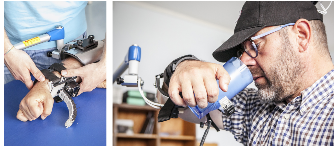
Figure 7.1: The proposed system: The Soft-SixthFinger works with the paretic upper limb to compensate for hand grasping functionality. The motion of the device is controlled by a wearable EMG interface embedded in a cap. The Passive arm support compensates the gravity force of the paretic upper limb.
