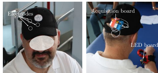
Figure 6.1: The frontalis muscle cap interface. The EMG electrodes are placed inside the cap at front side to be positioned on the patient’s forehead. The acquisition board is placed in a box on the back of the cap.
