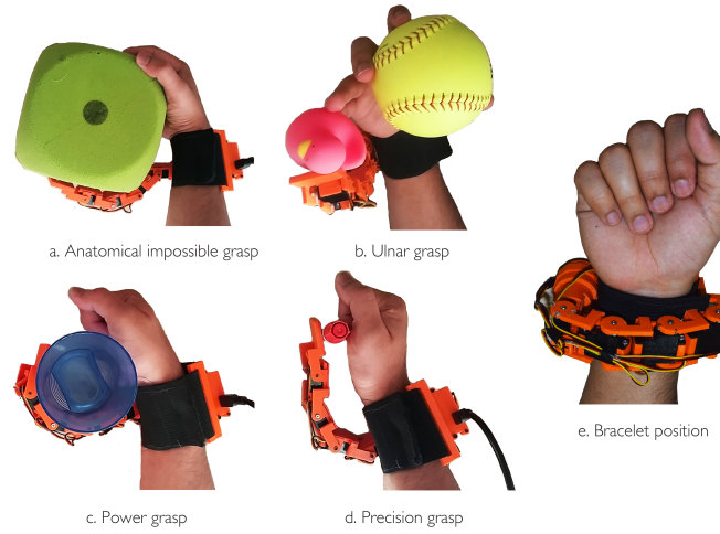
Figure 6.13: Examples of possible achievable grasps at working positions (a-d) and bracelet at rest position (e). In (a) and (b) the robotic finger coordinates with healthy hand to realize the anatomically impossible and ulnar grasp, respectively. While in (c) and (d) it interacts with paretic hand to realize power and precision grasp.
