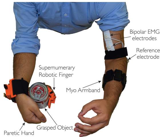
Figure 6.10: The complete system: the EMG interface on one arm while the supernumerary robotic finger on the other arm. Myo Armband is positioned on the forearm while the one channel interface is placed on the biceps muscle.
