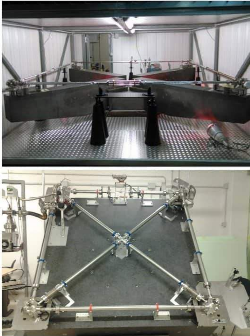
Fig. 1.7: GINGERino and GP2 italian ring lasers. Above: GINGERino, installed in the LNGS underground laboratory in Assergi (L'Aquila, Italy). Below: GP2, installed in the INFN laboratories in Pisa.
