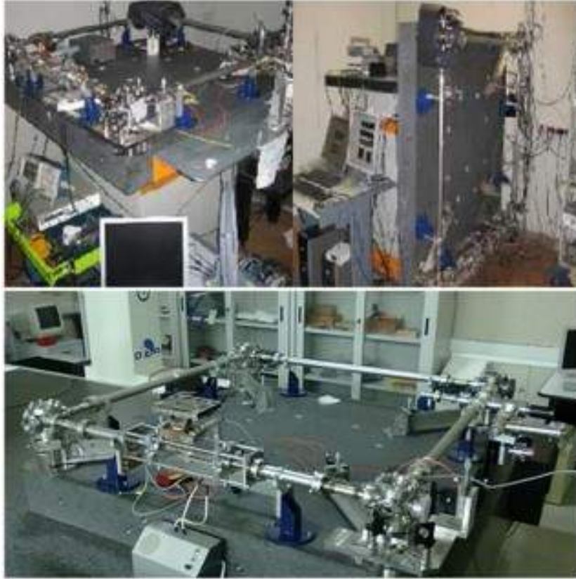
Fig. 1.6: G-Pisa ring laser. Above: horizontal and vertical configuration of G-Pisa inside the Virgo area. Below: its upgraded setup at the INFN laboratories in San Piero a Grado (Pisa, Italy).
