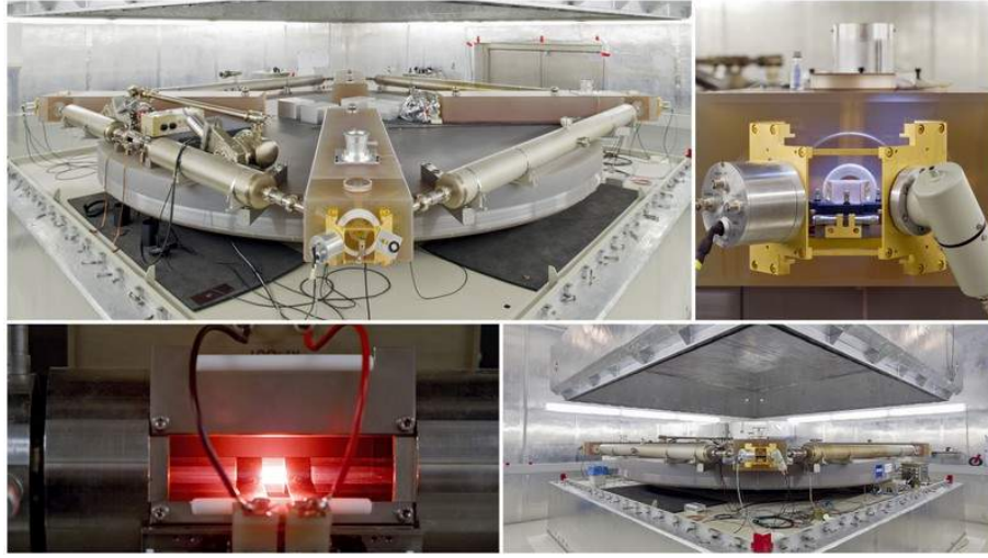
Fig. 1.4: The Gross Ring G. Above: overview of the semi-monolithic Zerodur structure whereon the optical cavity is installed (on the left); detail of the setup for Sagnac beat detection; a prism is used to combine the clockwise and counter clockwise beams. Below: pyrex plasma tube for radio frequency excitation of the gain medium (on the left); pressure stabilizing vessel enclosing the ring laser structure (on the right) [courtesy of U.K. Schreiber and A. Gebauer].
